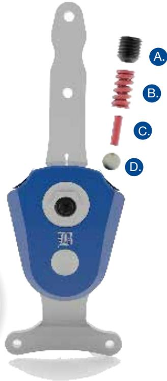
The Standard Resist and High Resist motion limiter pins are different sizes. To ensure maximum spring life, use only the silver (M3.2X11) motion limiter pin with the Standard Resist Spring (black) and the red (M3X10) motion limiter pin with the High Resist Spring (red).
