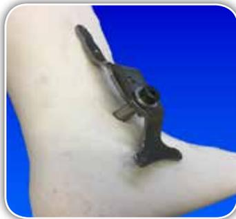
The Alignment Bushing fits into the Alignment Axis hole in the positive plaster mold.
