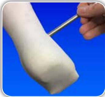
Set the ankle axis in the negative cast using the Alignment Axis in the Fabrication Tool Kit, and fill the mold. Strip the mold and remove the Alignment Axis from the positive mold.
